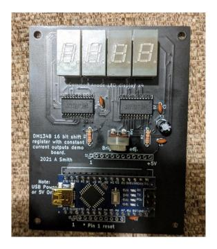
Thanks for purchasing this item. This PCB consists of two DM134B 16 bit shift registers with open drain outputs and constant current sinking capability. Sinking current is set via a single resistor on each chip. When the brightness is set at maximum this is approximately 20mA and at minimum brightness approximately 2mA.
